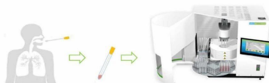
Figure 1 Automated RNA extraction workflow: in a fume hood the dry swabs need to be equilibrated in a physiological/isotonic solution (e.g. PBS) followed by a short incubation. From this liquid 300µL is transferred as sample into a deep-well-plate followed by the addition of 4µl Poly(A) buffer, 10µl Proteinase K and then 300µl Lysis buffer before starting the automated extraction.
